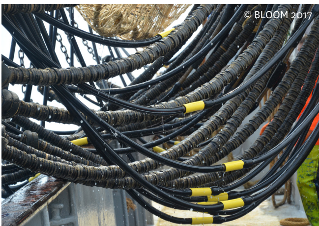
Focus on cables on an electric 'pulse' trawl.
